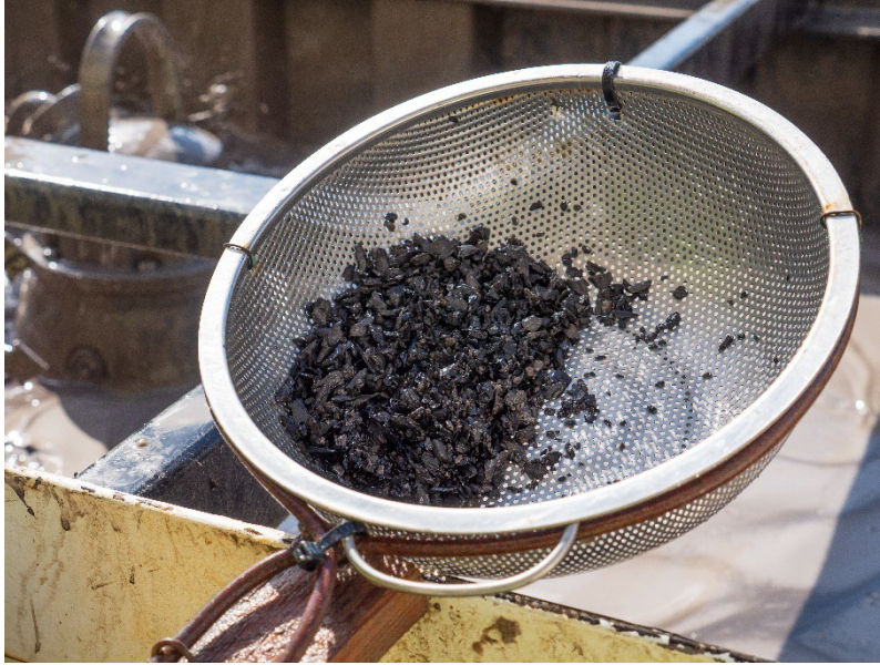
Figure 10: Rock Cutting Analysis. Here, dark and soft claystone cuttings can be observed
