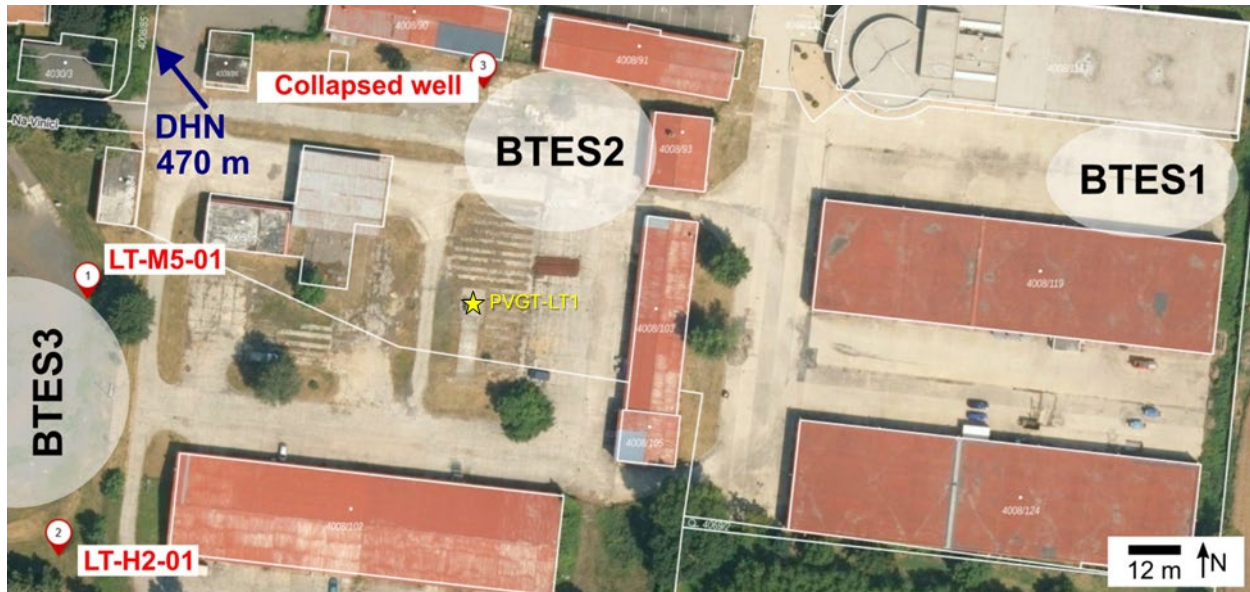
Figure 1: Wells drilled in the PUSH-IT project (1 to 3, red), old exploration borehole PVGT-LT1 (yellow), planned BTES fields in the SYNERGYS project (black) and potential connection to DHN (blue).
